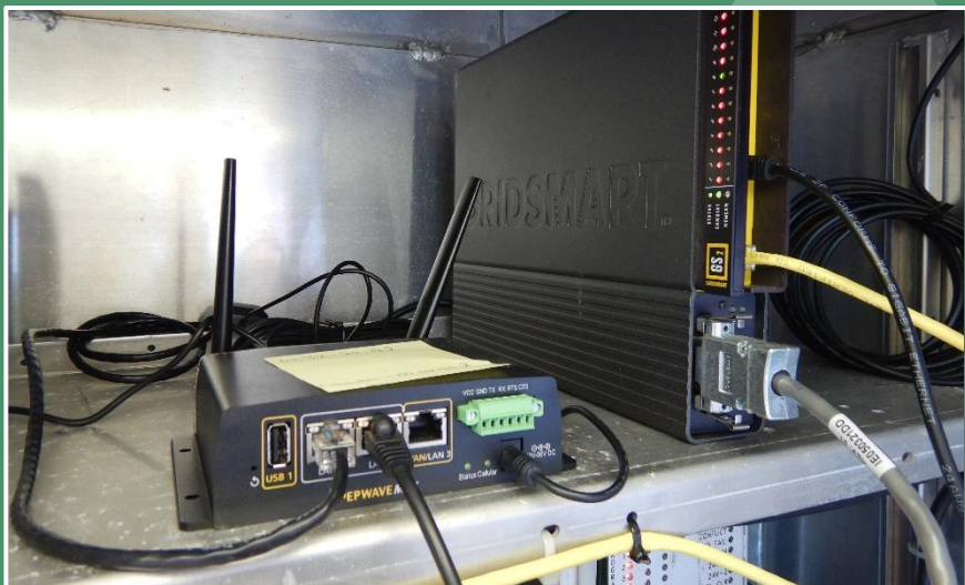
Cellular modems provide routing capabilities to act as network communication devices at locations where switches are not present and multiple network-enabled devices are required; maximum of three (3) RJ-45 ports. (Brevard County)
