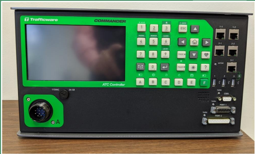
Trafficware (now Cubic ITS) COMMANDER ATC unit, NEMA TS-2, Type 1 model; shown in bench testing phase.
