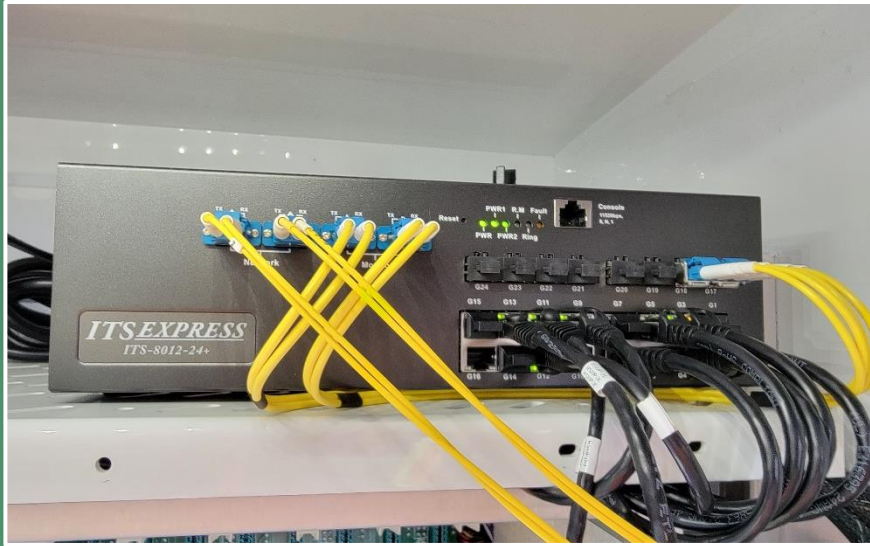
Each model of managed field Ethernet switch (MFES) includes a variety of ports for fiber optic medium (e.g., SFP) and copper (e.g., RJ-45). (Seminole County)
