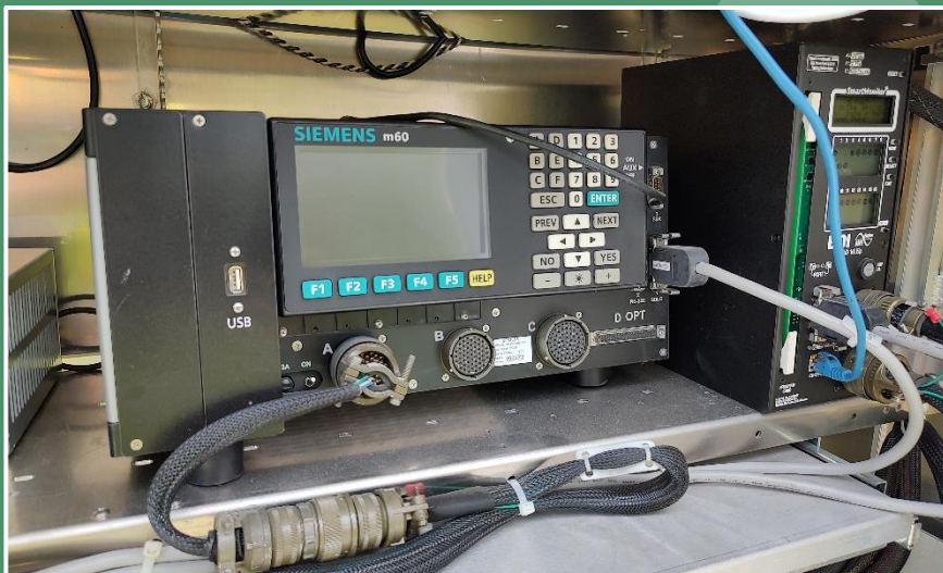
Siemens (now Yunex Traffic) m60 ATC unit, TS-2 Type 2 model, operated as Type 1 ("A" connector only). (Marion County)
