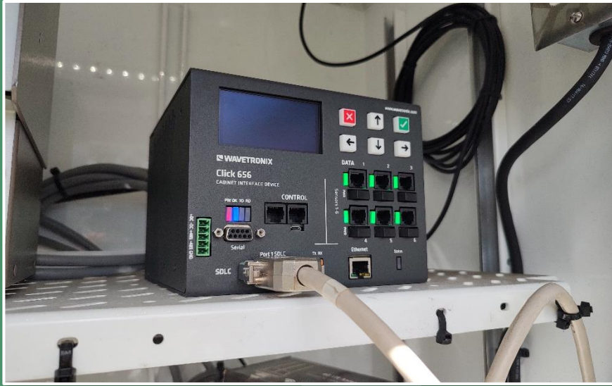
Example in-cabinet processor with capacity for six (6) unique microwave vehicle detection system sensors with SDLC bus connection. (Lake County)
