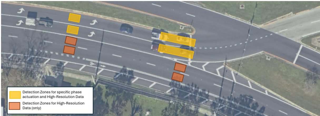
Figure 10: Example of presence detection at a free-flow intersection
