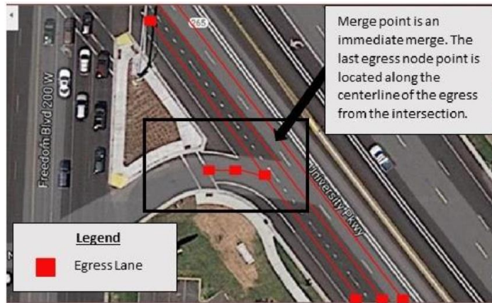
Figure 14: Example Egress Node Placement for an Intersection Where the Merge Point is an Immediate Merge
