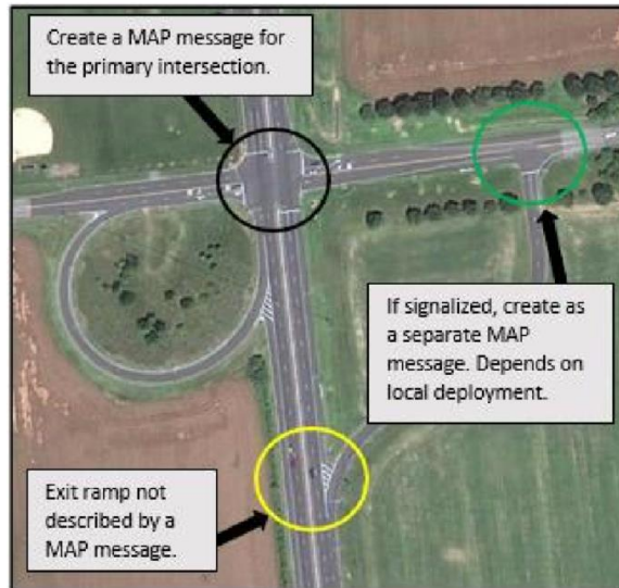
Figure 18: Aerial View of Jug Handle Intersection
