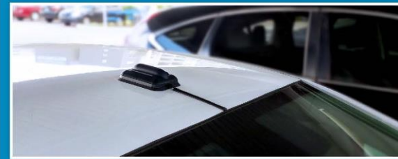
Single antenna on the roof of a sedan
