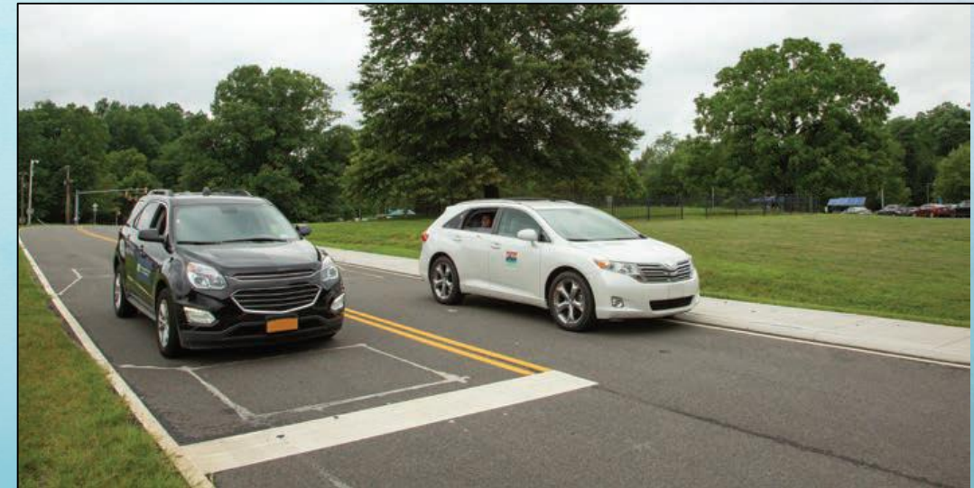
THEA vehicle (white car) passing stationary NYCDOT vehicle at test track without triggering forward collision warning alert.
