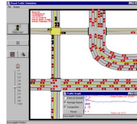
Mesoscopic Simulation for Realtime 30 Minute Forecasting
