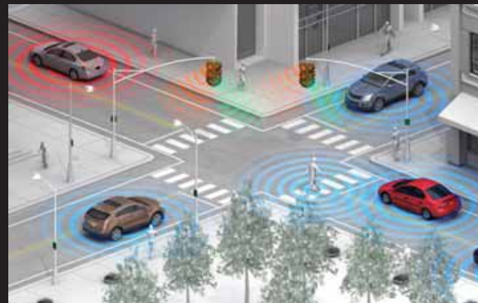
Illustration of warning messages about pedestrians' red-light crossing with the connected vehicle technology
