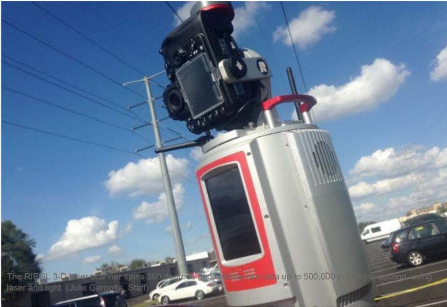
The RIEGL 3-D laser scanner spins 360 degrees and collects raw data up to 500,000 points per second, using laser and light. (Julie Gargotta, Staff)
